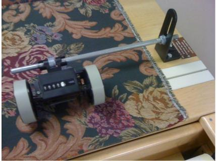
Fabric should be pulled past cutting groove before TRUMETER is flipped to measuring position. This allows for accurate and straight cuts.
