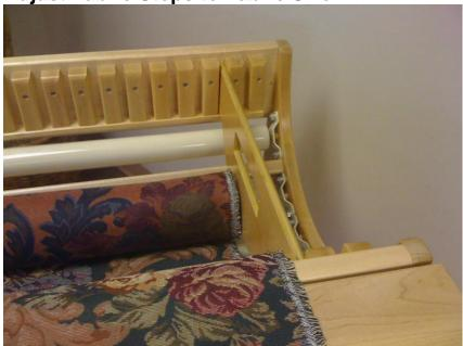
Put the fabric stop in the position that lines the fabric straight in the hopper and corresponds with the size of the fabric and/or tube.
