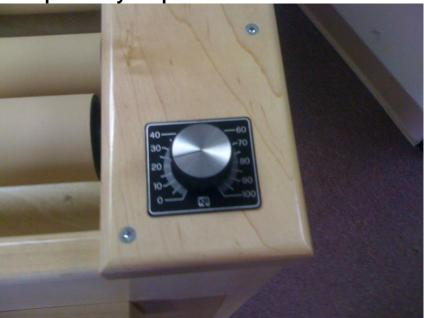
Set speed by turning the speed control knob.
