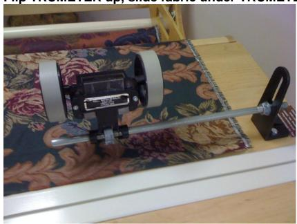
TRUMETER Should flip up so bottom of TRUMETER is exposed at this stage of rerolling.
